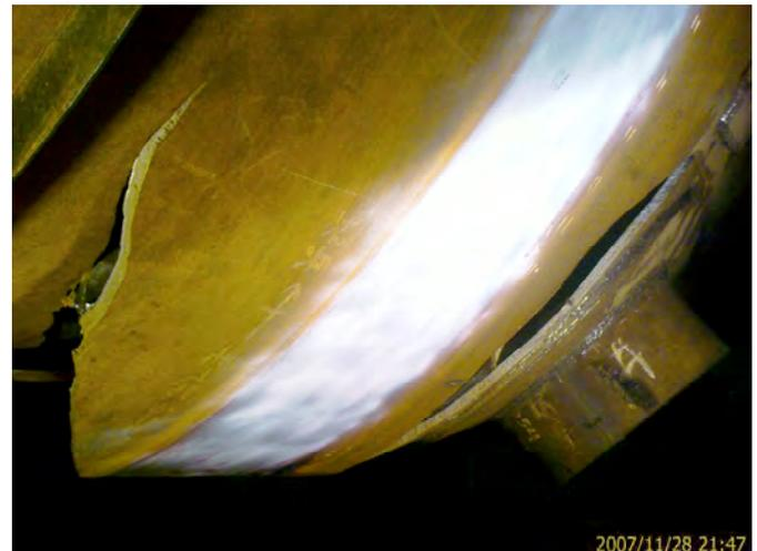
This vessel was manufactured by Nanjing Yuchuang Co. in China and the plate was of Chinese origin. Unfortunately, this is another example of serious equipment/material failures with equipment being sourced out of the rapidly developing economies such as China, Eastern Bloc and others. These examples are becoming almost a weekly occurrence now and are exhibiting failure modes not seen in the manufacturing economies since the 1930's.
